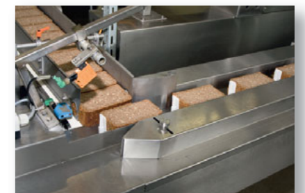
The freshly baked bread is cooled, then cut into slices and automatically transferred to the packaging machine..
